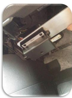
Plug on the lock and screw it together
