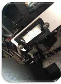
Bolt the OBD housing & jack together with the housing
